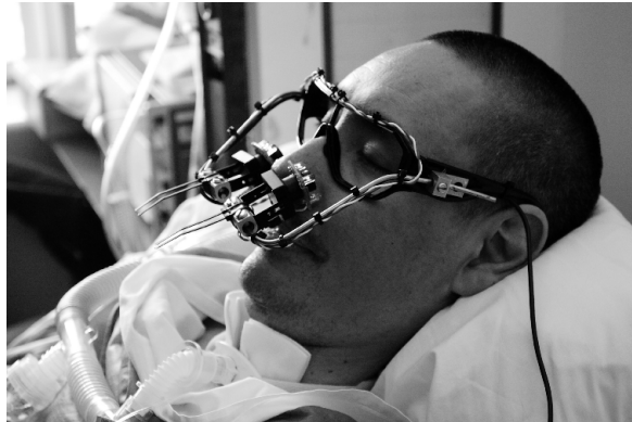
Fig. 4.3: Tempt using the Eyewriter open source eye-based HCI
