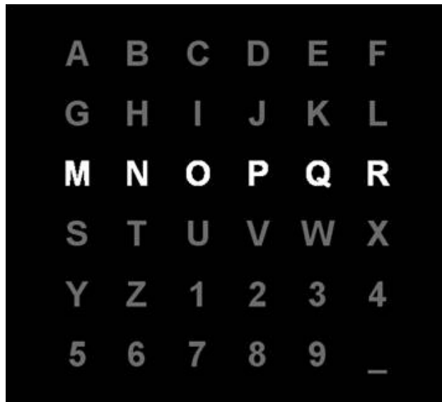
Fig. 5.48: A typical square setup used in P300 applications
