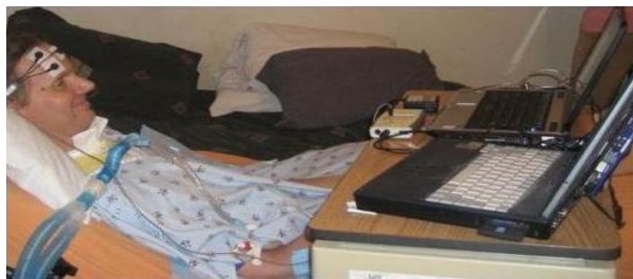
Fig. 4.2: Neuroswitch system being used by a LIS patient
